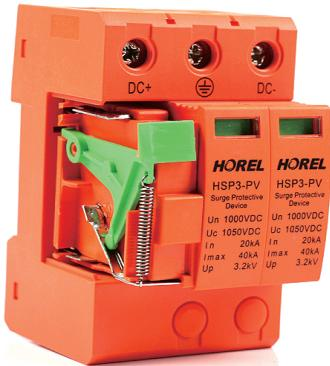
HSP2-PV(HSP3-PV) surge protection device is a surge protection specialized for solar PV generation system, mainly used in generation system with voltage DC1000V and the maximum discharge current capacity 40kA.
